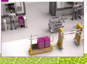
Logistics systems such as BLOKSMA taxi or portal wagons ensure that only as much material is provided in assembly and manufacture as is necessary, or as much as has already been used.
